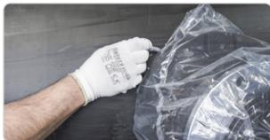
**5. Place the fitting in the bag and re-measure the welding zone. Check if the entire zone is well prepared (no line has been missed)**
