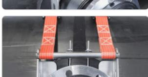
**e. Tighten the belts evenly from each side using tightener, make sure that the belts are placed equally at the end of the installation roller**
