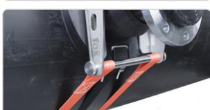
**c. Put the clamping tool FOXGRIP L on the saddle with installation roller N° 1**
