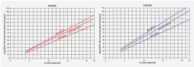
NOTE. Thermal outputs according to thermostatic chamber tests. Outputs refer to actual surface of the panel.
