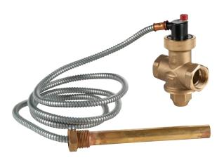
The R144ST thermal safety relief valve is a device that limits the temperature of the water in multi-fuel or solid (nonpulverized) fuel generators equipped with a built-in storage tank or emergency heat exchanger (for immediate cooling). When the calibration temperature is reached, the valve begins discharging the right amount of water to keep the generator temperature within the safety limits.
