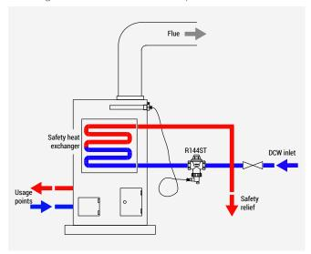
**A WARNING.** The thermal drain valve is intended to avoid exceeding the maximum allowed temperature in the system; according to the norm 4.6.1 EN 12828, the installation of a safety device preventing overheating above the maximum allowed temperature is required.
