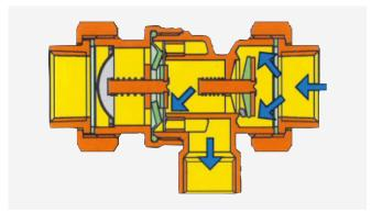
In the event of back pressure or depression upstream, the drain will open and, if the second check valve is obstructed for any reason, the polluted water is expelled.
