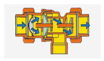
The transit sections are calculated so as to limit the pressure loss of the backflow preventer, thereby guaranteeing optimum flow rates.
