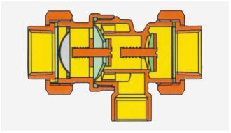
In static conditions, the check valves are closed.
