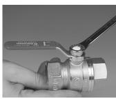
1) Unscrew the nut with the appropriate key.
