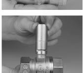
3) Install the cylindrical extension of the pin, that must be fitted in on the stem of the ball valve, paying attention to the opening direction.
