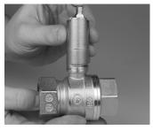
**4)** On the stem of the ball valve, screw the central pin of the R749T universal extension. and use the lever of the ball valve, to screw deeply.
