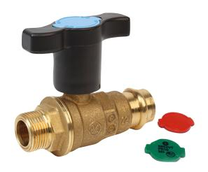
Ball valve, with male threaded-press connections (for copper pipe complying with EN 1057; for stainless steel pipe complying with EN 10217-7 and EN 10312; for carbon steel pipe complying with EN 10305-3), for pipes with high insulation thickness, specific for domestic water. Full port.
