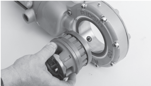
Figure 4 – Installing Die Heads into 700 Power Drive
