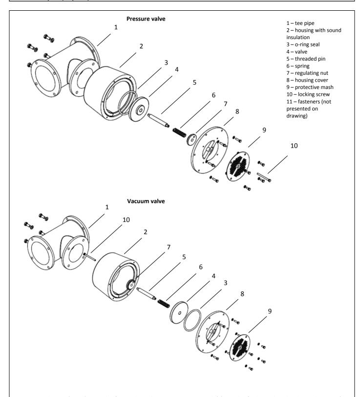
Construction elements (1, 2, 8) are made of painted cast aluminium. Protective mesh (9) is made of galvanized steel. Valve working parts (4, 5, 6, 7) are made of steel. Fasteners (10, 11) are made of galvanized steel, and seals (3) are made of NBR.
